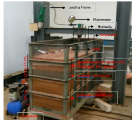
Fig. 4: The arrangement of the physical model of road base layer test
